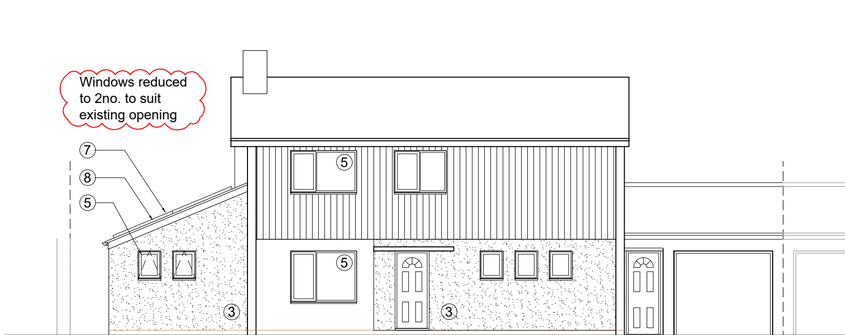
Front Elevation - East Facing
