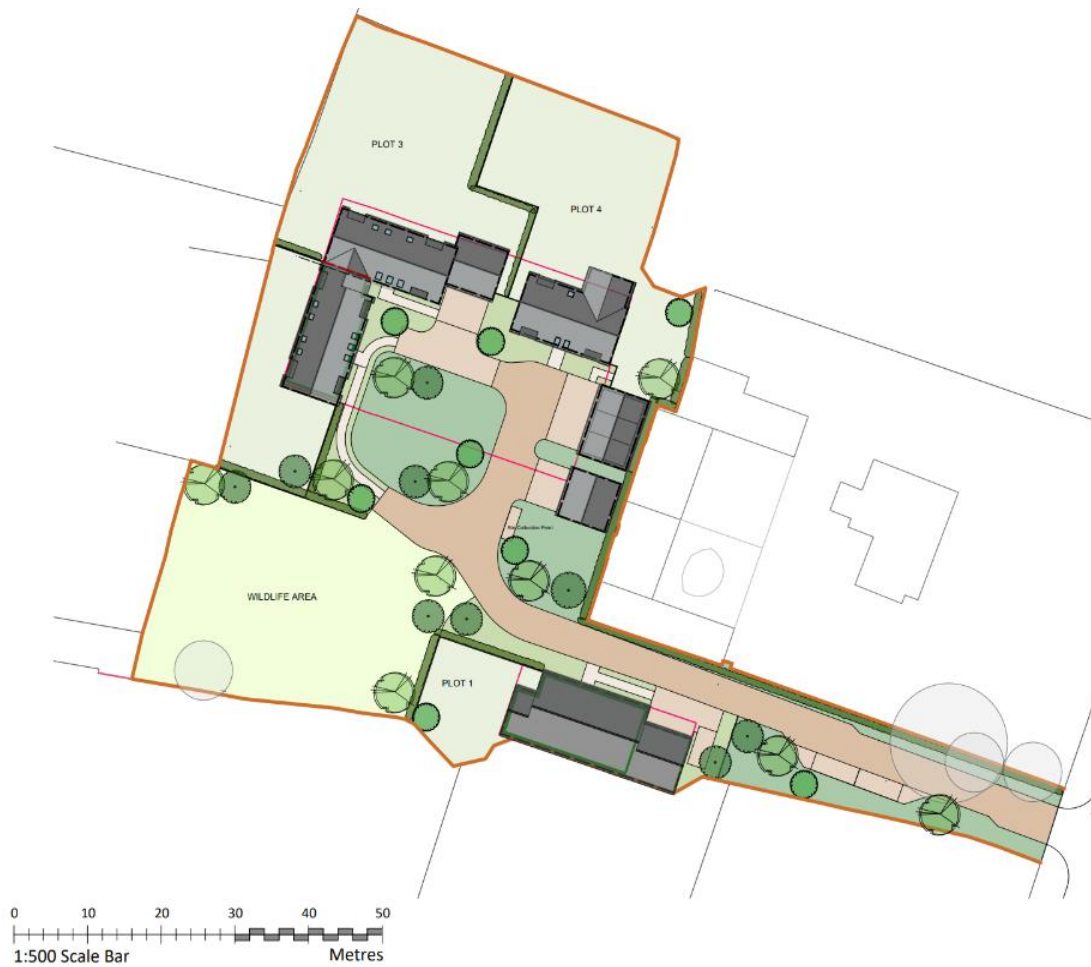
Figure 2 – Proposed Site Layout Roof Plan – for scaled version please see ref: 224420-PL-S-00-102
