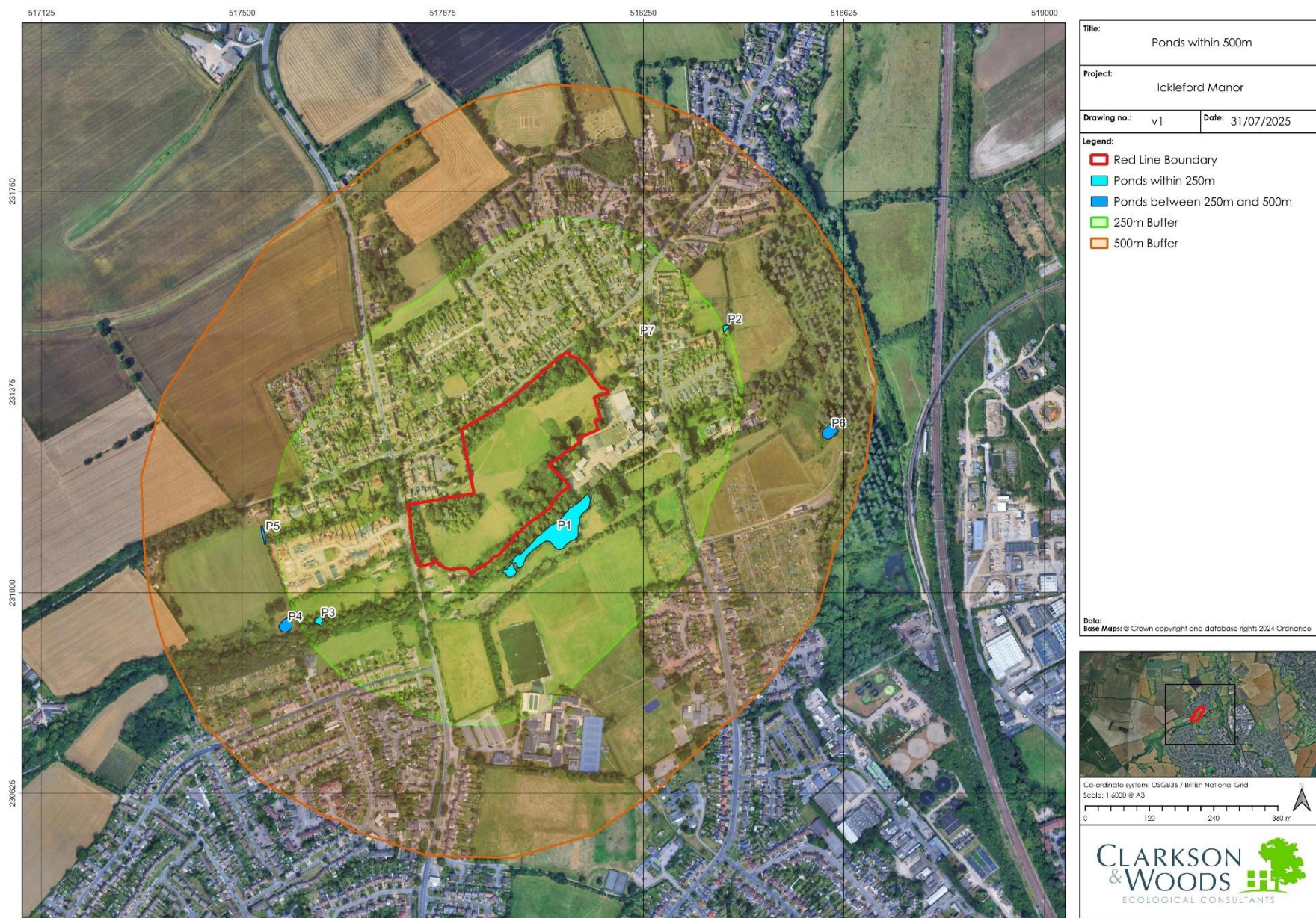
Figure 7: Ponds identified within 500m of the Site Boundary
