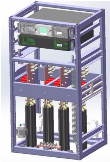
Figure 6-11 Elementa bus bar DC power connection
