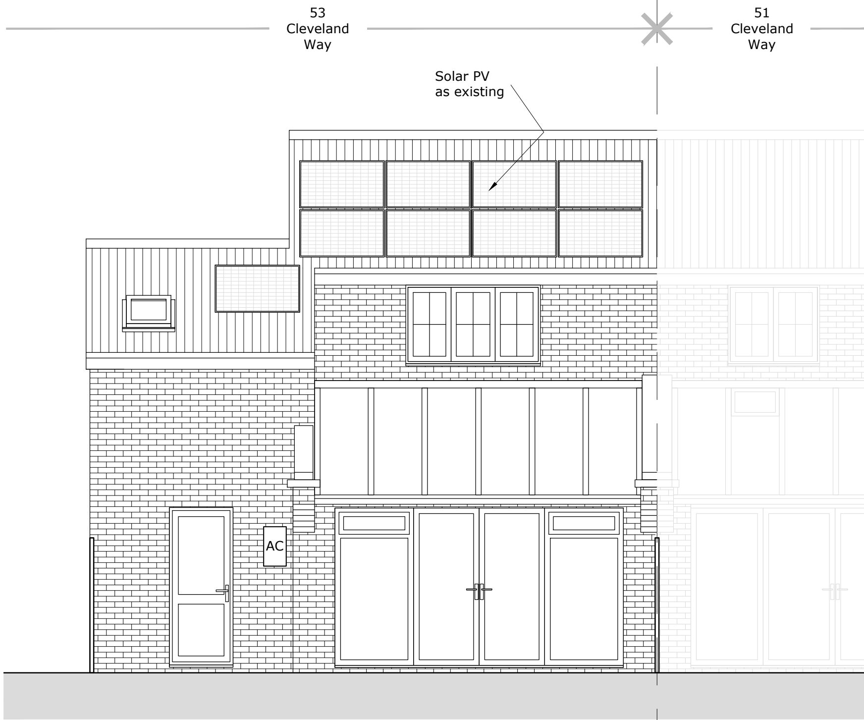
South Elevation as EXISTING 1:50
