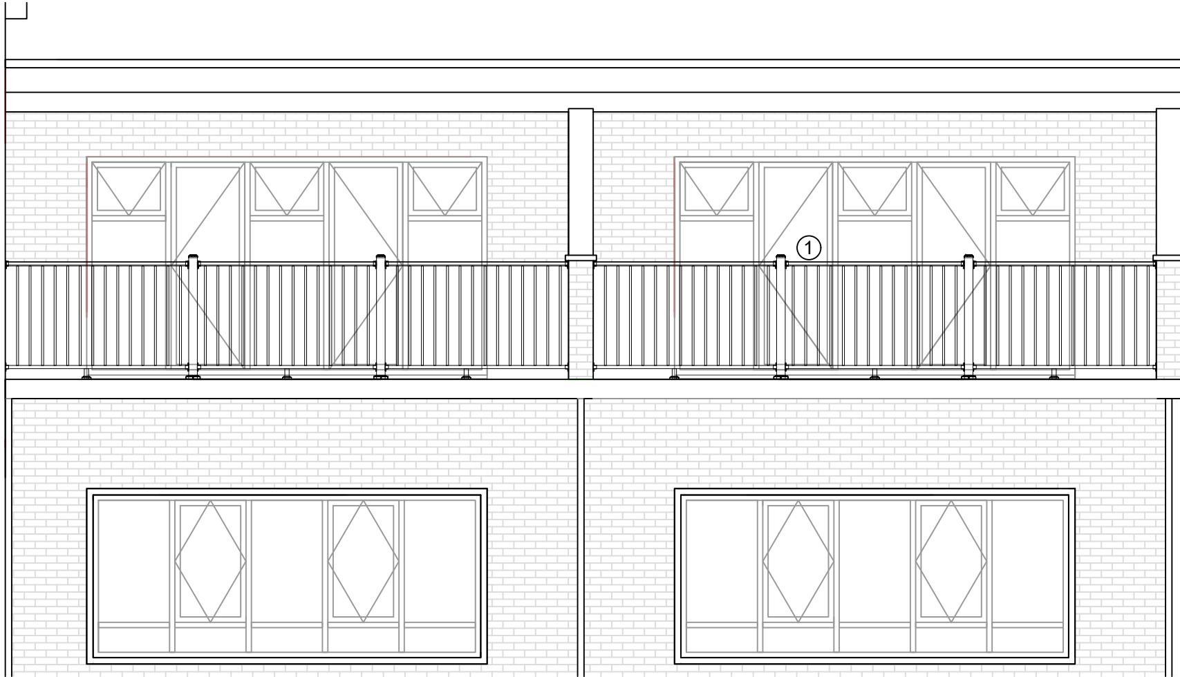
BALUSTRADING ELEVATION AS PROPOSED 1:50
