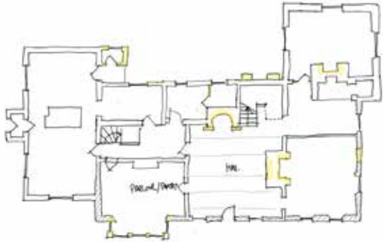
Late 19th early 20th Century New rear porch, fireplace alterations to the hall, front reception room and rear office. New bay window, rear buttressing and infills.
