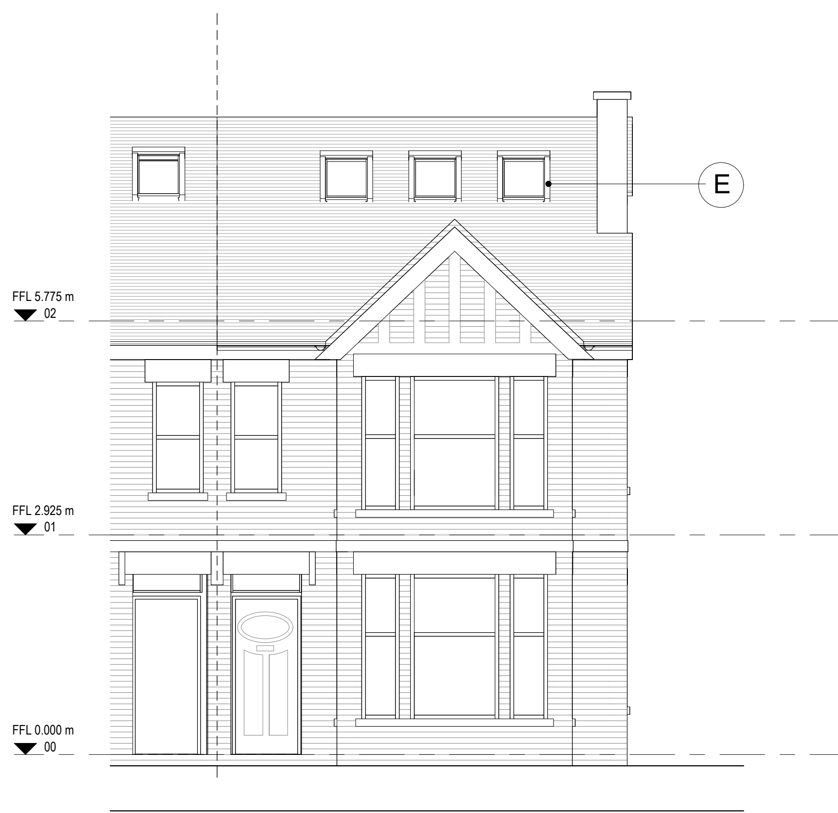
3 Front Elevation (South-West) 1 : 50
