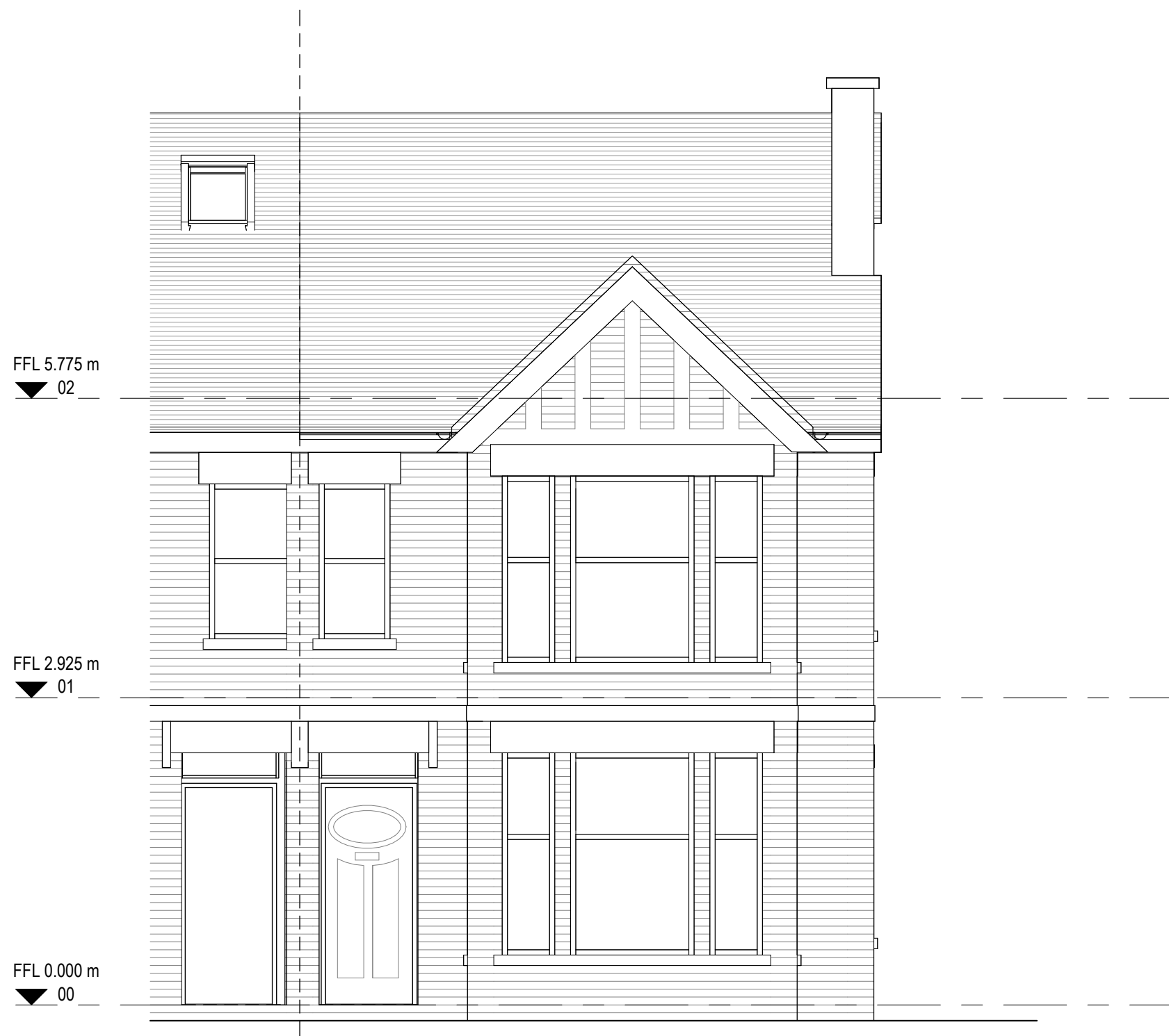
3 Front Elevation (South-West) 1 : 50
