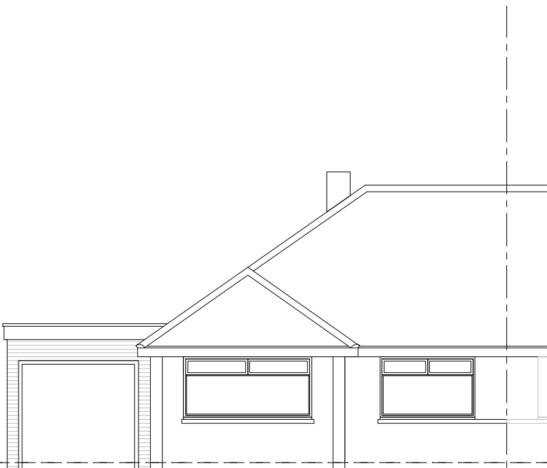
PROPOSED FRONT ELEVATION SCALE 1 : 100 Showing new and converted garage.
