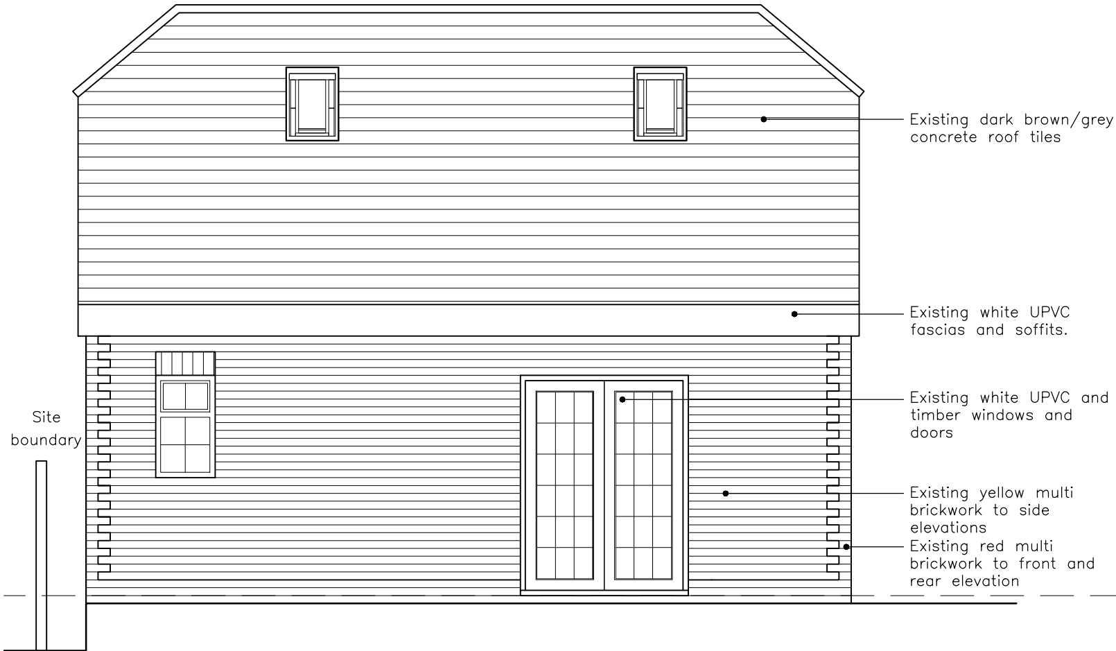
EXISTING ANNEXE SIDE ELEVATION 1:50@A1
