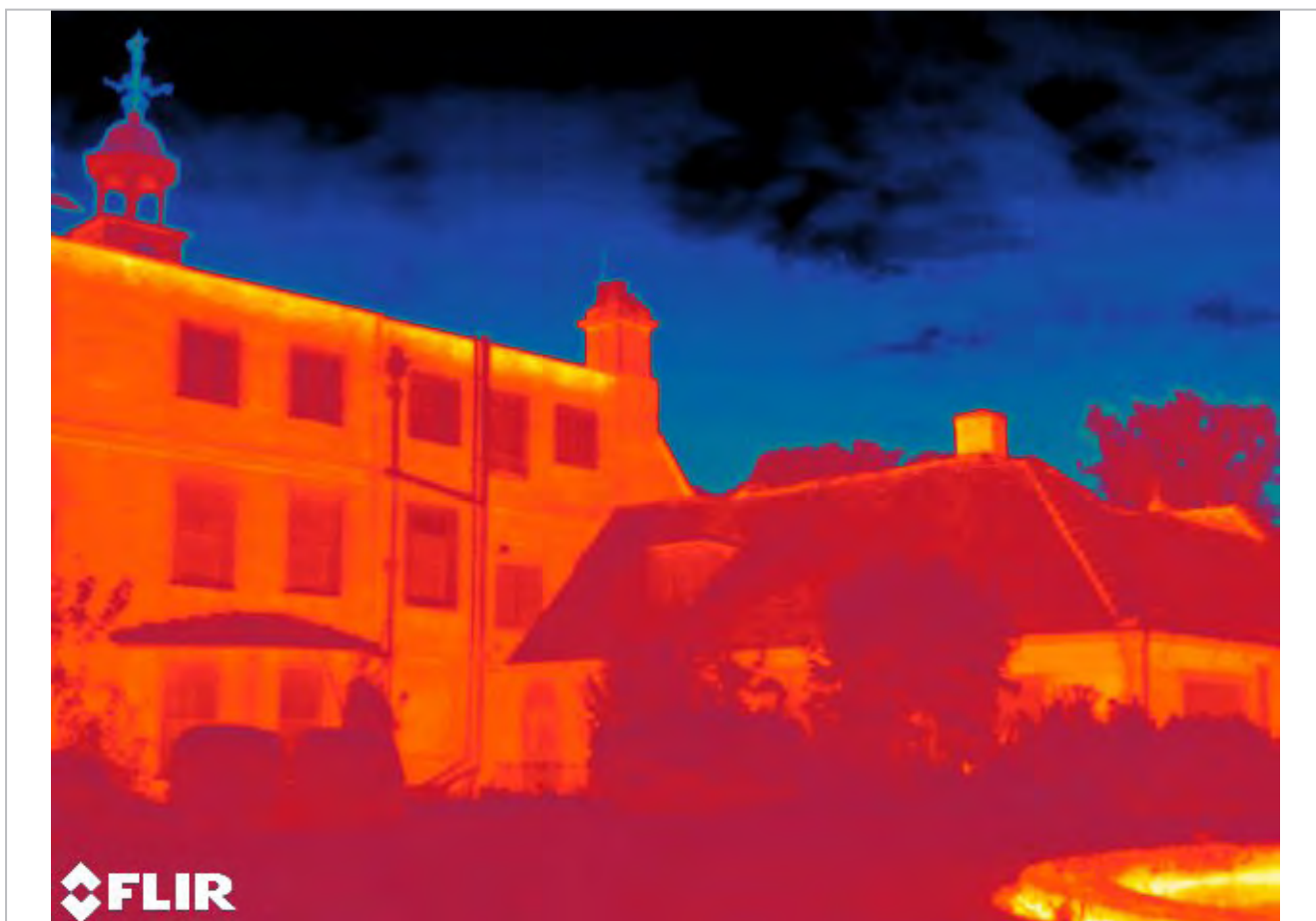
FLIR T540 (464 x 348 pixel resolution) with 42 degree lens = bat in flight detection distance of 51 m. Camera located 30 m from furthest point of building
