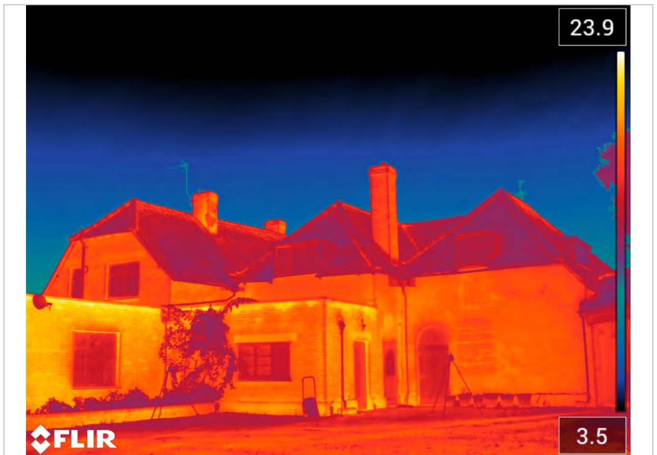
FLIR T1020 (1024 x 768 pixel resolution) with 45 degree lens = bat in flight detection distance of 104 m. Camera located 38 m from furthest point of building
