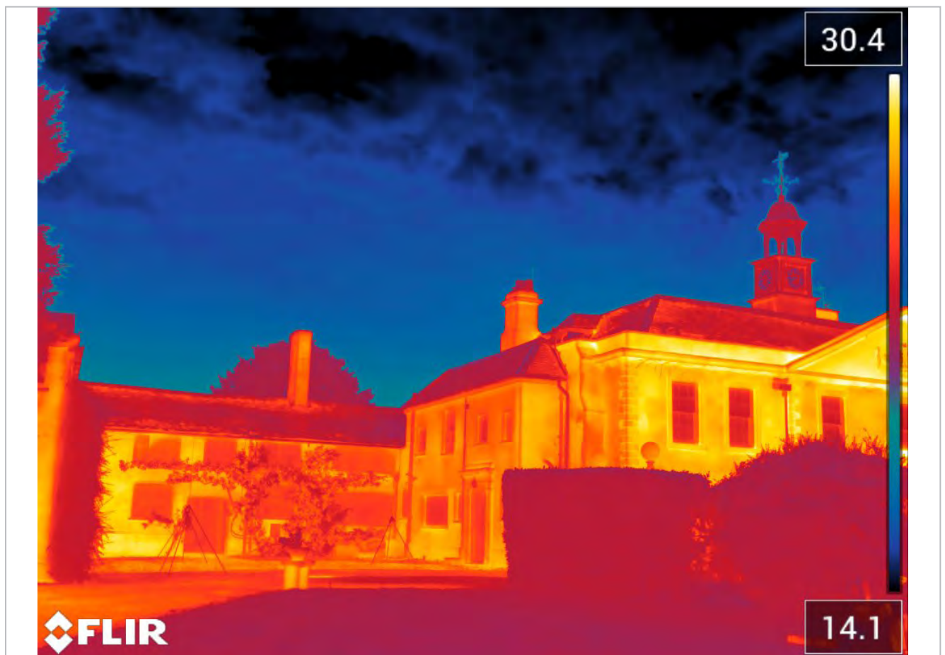
FLIR T1020 (1024 x 768 pixel resolution) with 45 degree lens = bat in flight detection distance of 104 m. Camera located 43 m from furthest point of building
