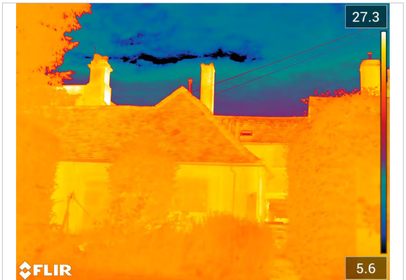
FLIR T1020 (1024 x 768 pixel resolution) with 45 degree lens = bat in flight detection distance of 104 m. Camera located 30 m from furthest point of building
