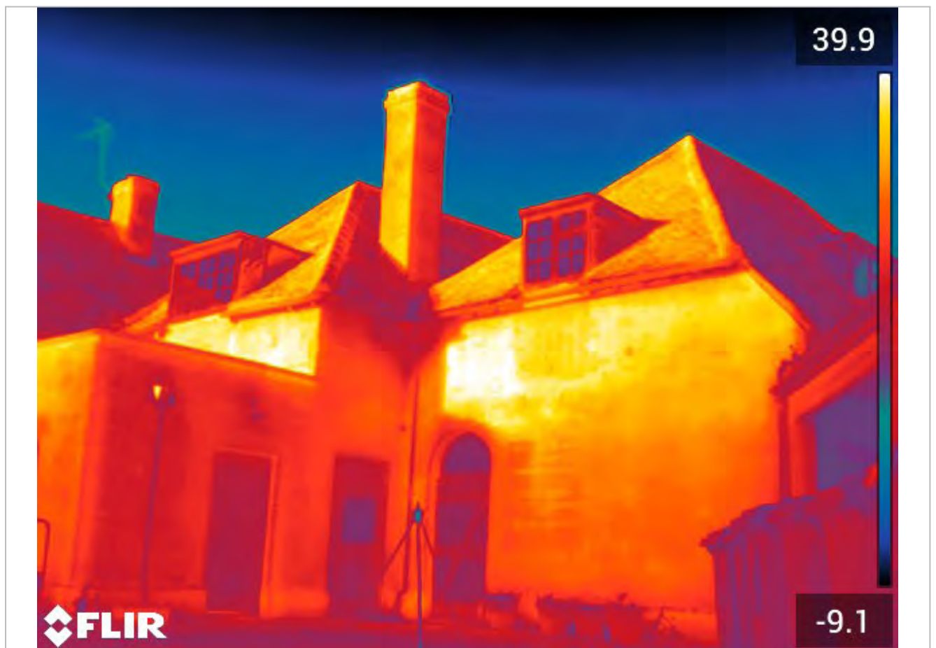
FLIR T540 (464 x 348 pixel resolution) with 42 degree lens = bat in flight detection distance of 51 m. Camera located 19 m from furthest point of building
