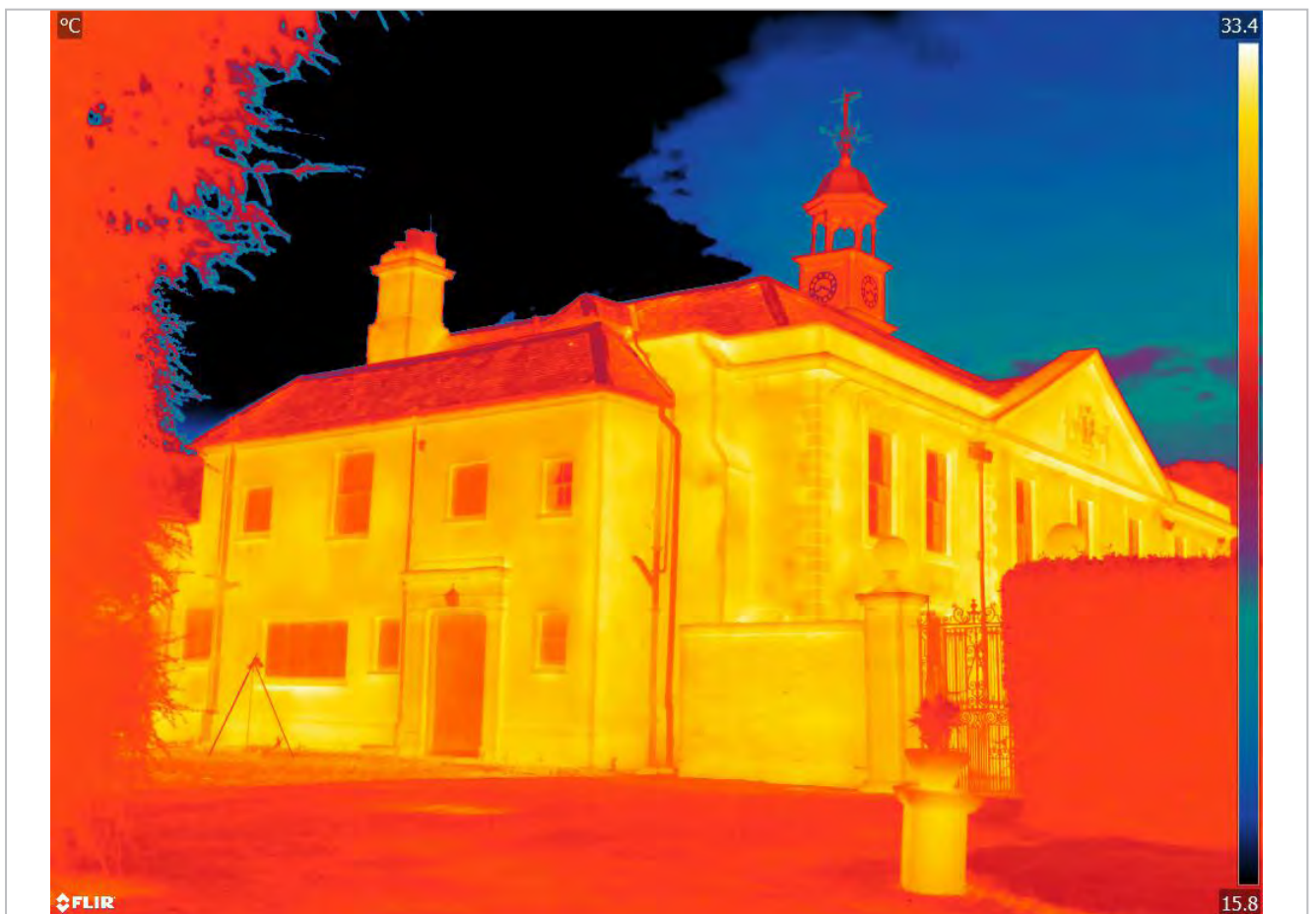
FLIR T1020 (1024 x 768 pixel resolution) with 45 degree lens = bat in flight detection distance of 104 m. Camera located 28 m from furthest point of building
