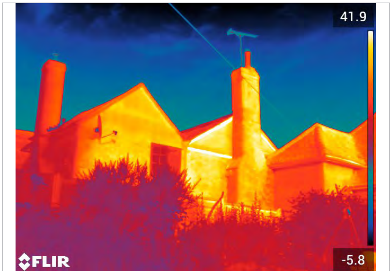
FLIR T860 (640 x 480 pixel resolution) with 42 degree lens = bat in flight detection distance of 66 m. Camera located 19 m from furthest point of building
