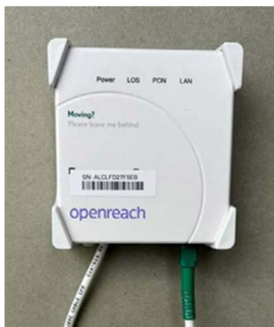
Figure 8.4 – Openreach ONT equipment
