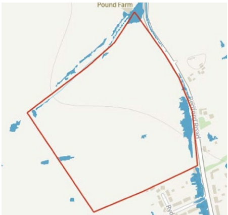
Extent of 1 in 100 Year Surface Water Flooding (Medium)
