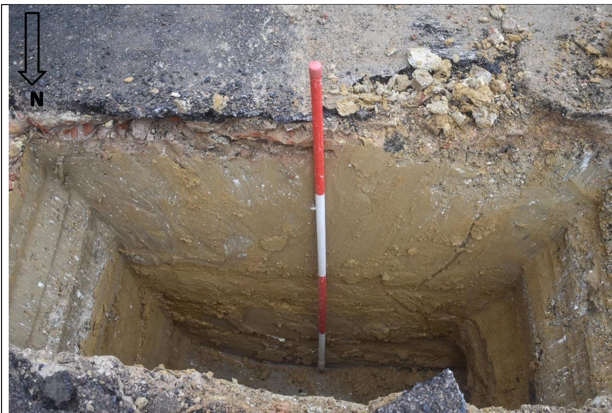
Plate 2: Geotechnical test pit, looking south, showing the natural superficial geology and the overlying tarmac hardstanding and its bedding material (scale 2m)
