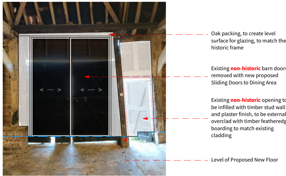
D. New Glazing to Dining Area in Existing Opening Bay 3
