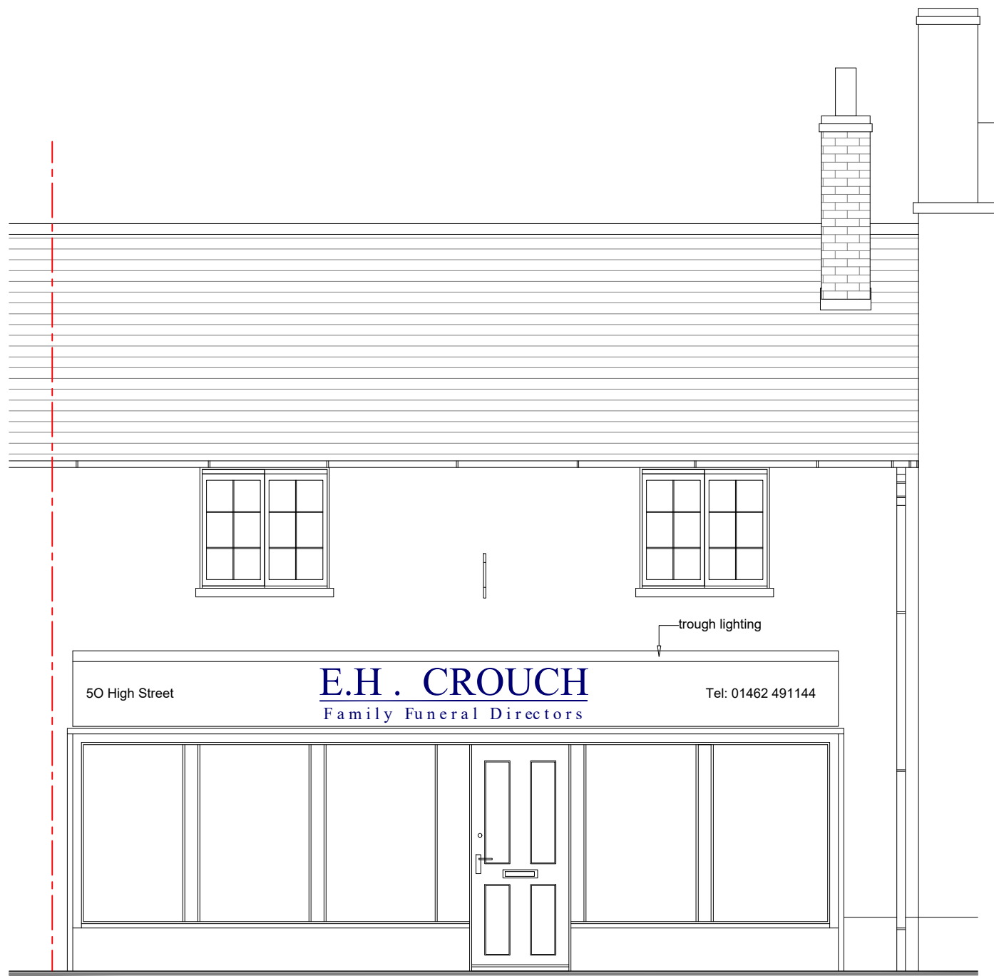
EXISTING NORTH/EAST FACING ELEVATION Scale 1:50
