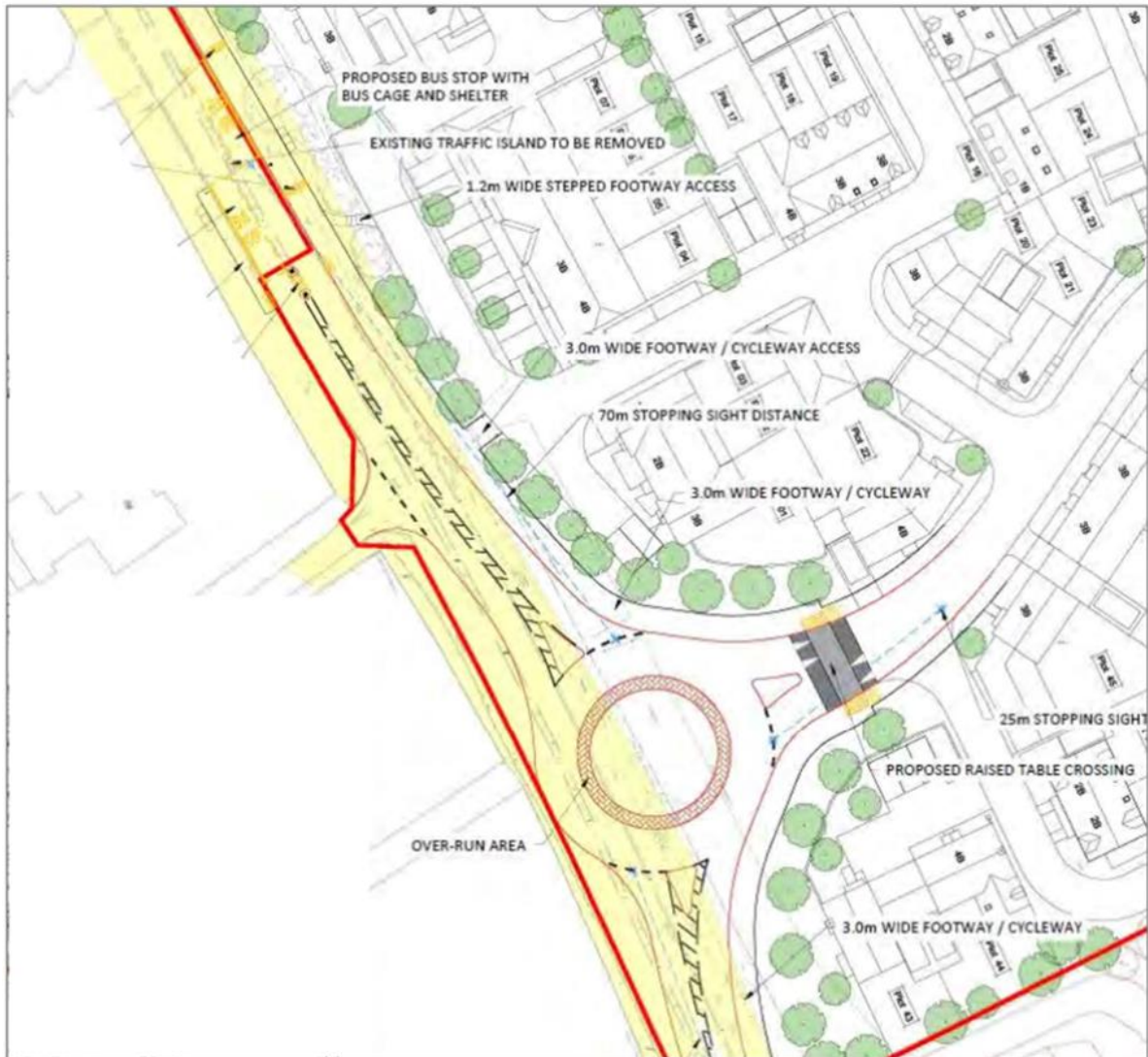
Figure 3-7 - Shared Footway/ Cycleway at Pound Farm Development
