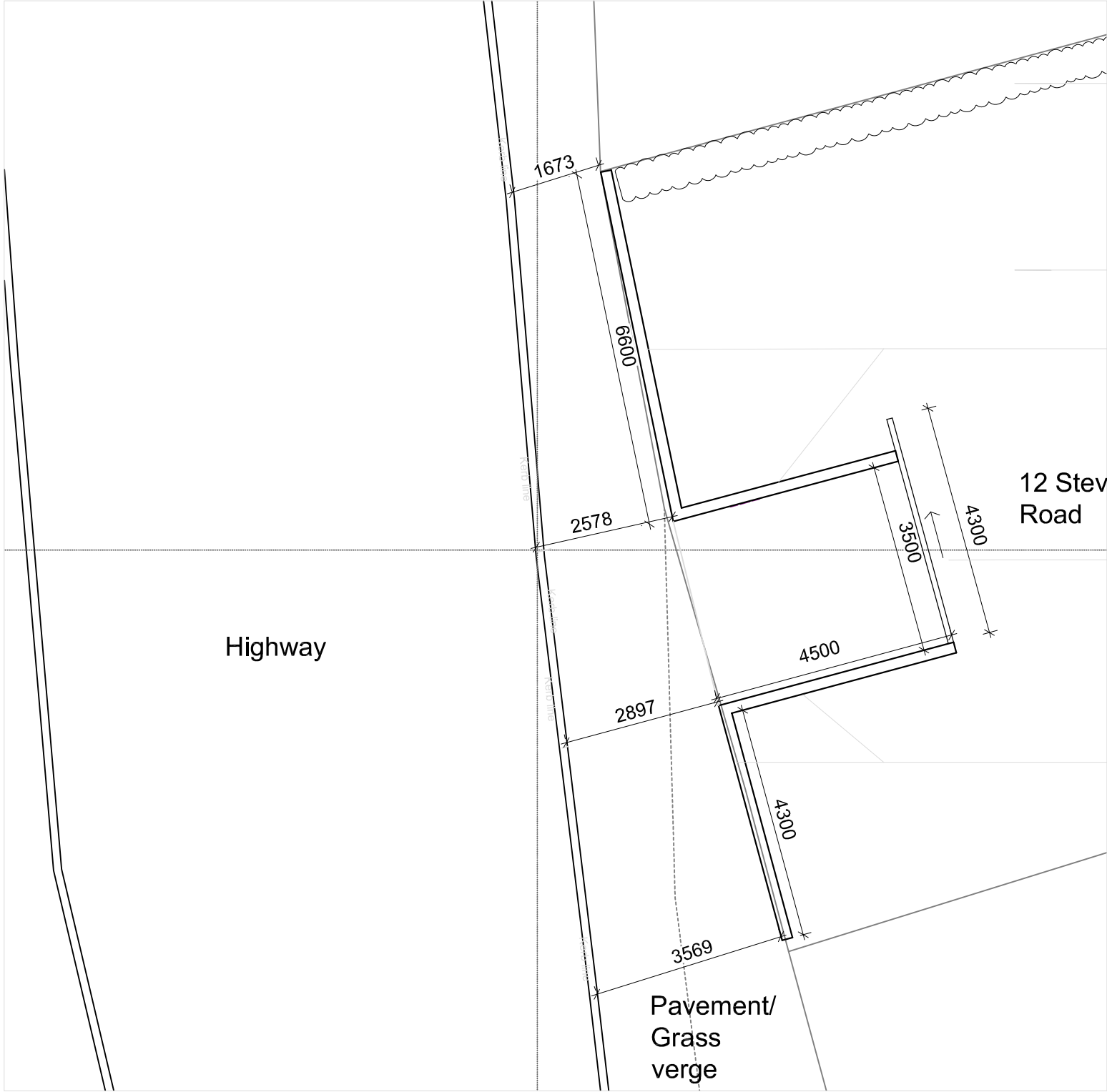
Proposed PLAN - Brick Garden Wall and Gate Scale 1:100 @A3
