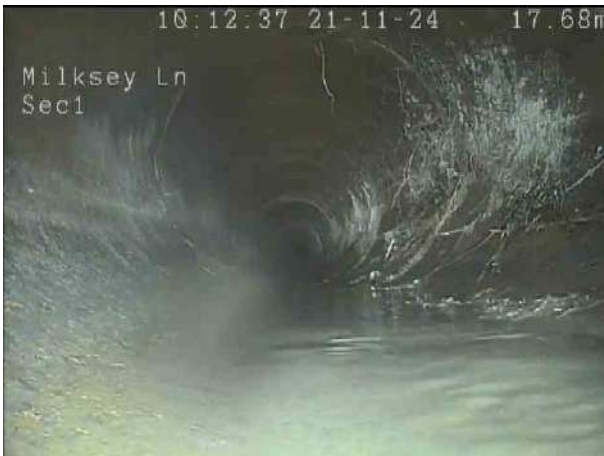
b2a526c9-151c-40f6-809e-3401277c87f8.png, 00:00:51, 18.20 m Roots, fine at joint, start
