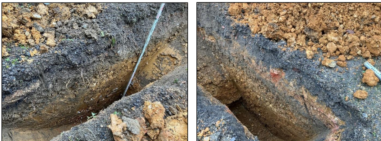
Figure 6-A: TP01 (left) and TP05 (right) showing gravels over clay Made Ground over Clay-with-flints Formation.
