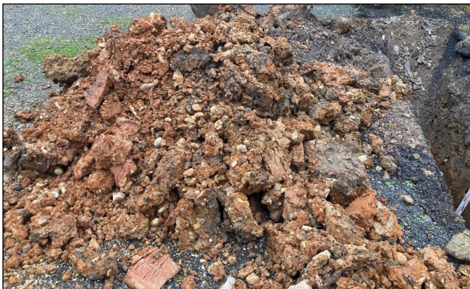
Figure 6-D: Clay-with-flints Formation excavated from TP02
