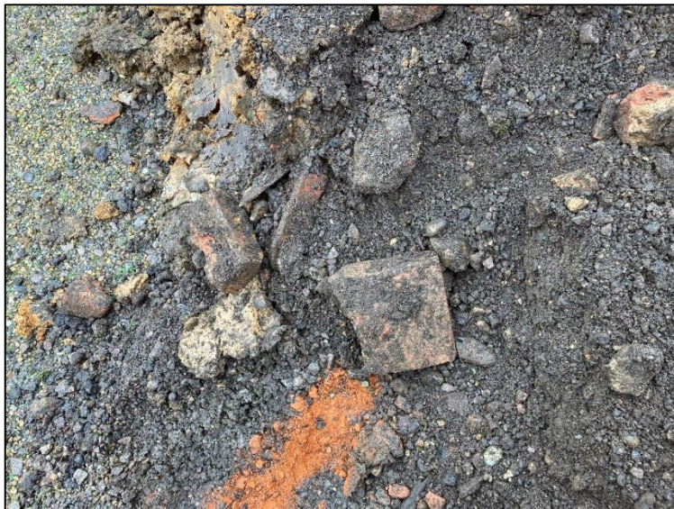
Figure 6-C: Made Ground excavated from TP03
