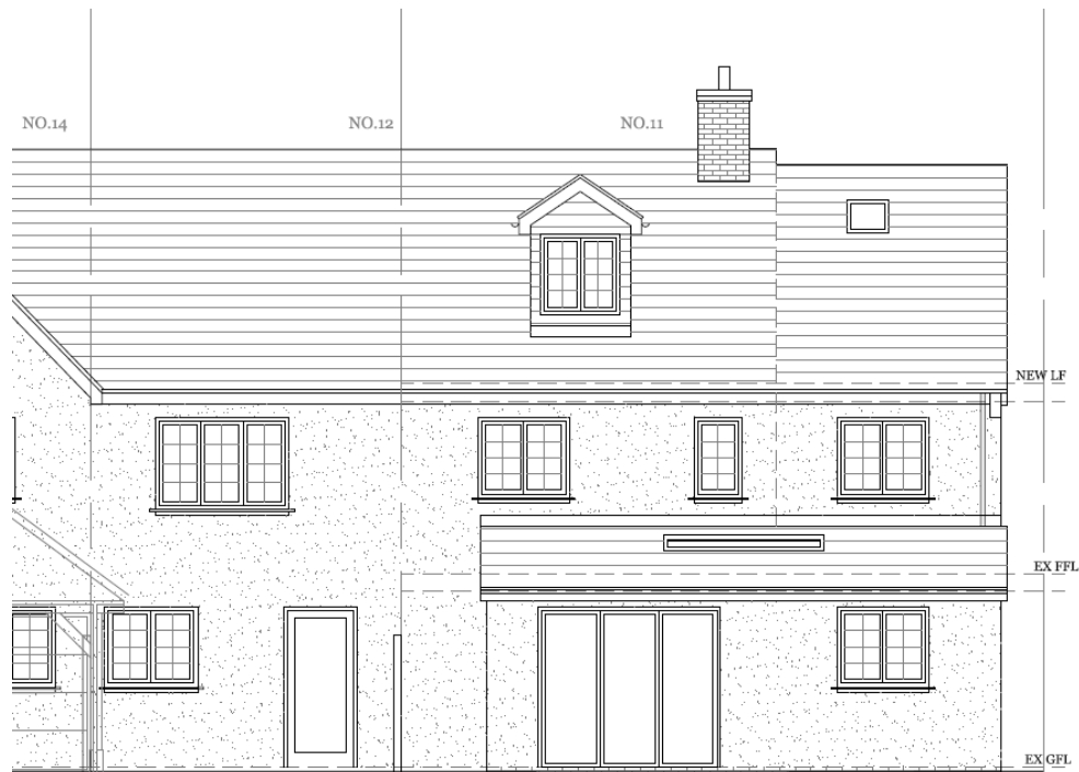
Fig 2. Rear Elevation with neighbouring context.
