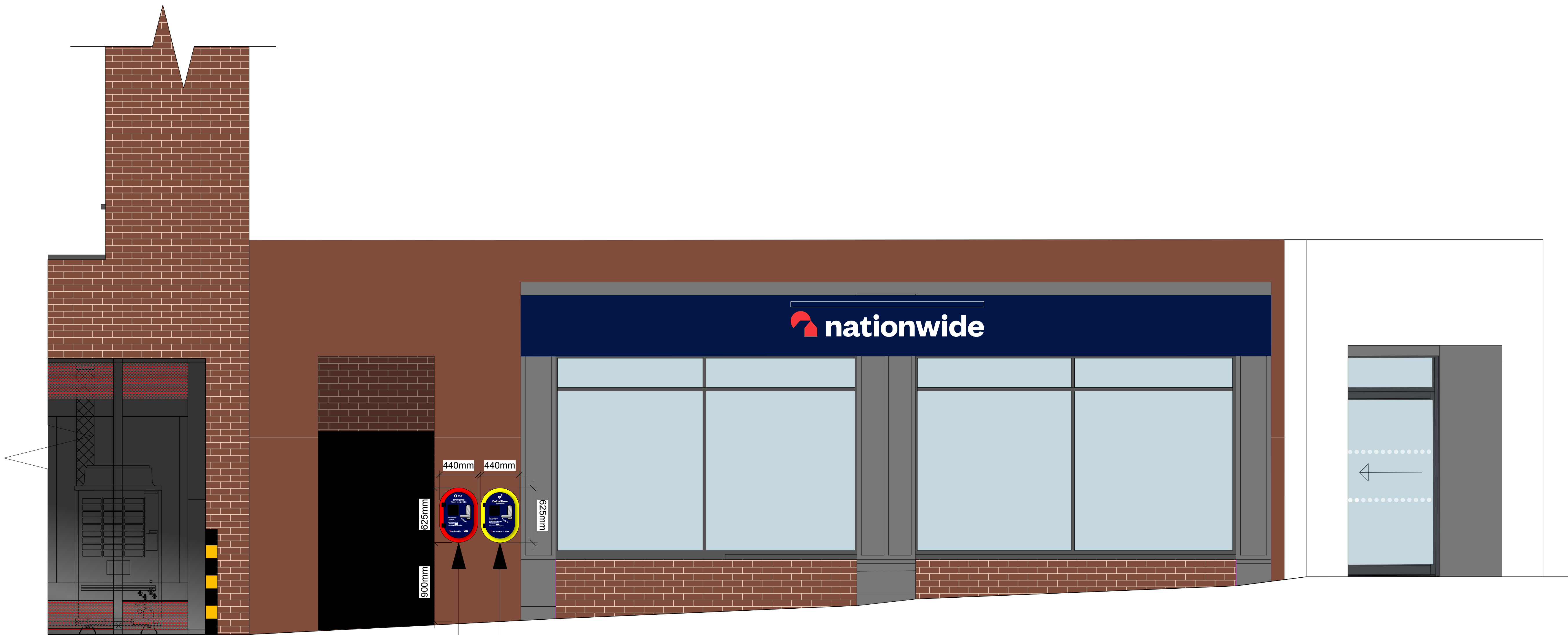
NEW BLEED KIT CABINET INSTALLED NEW DEFIBRILLATOR CABINET INSTALLED WITH INTERNAL ILLUMINATION
