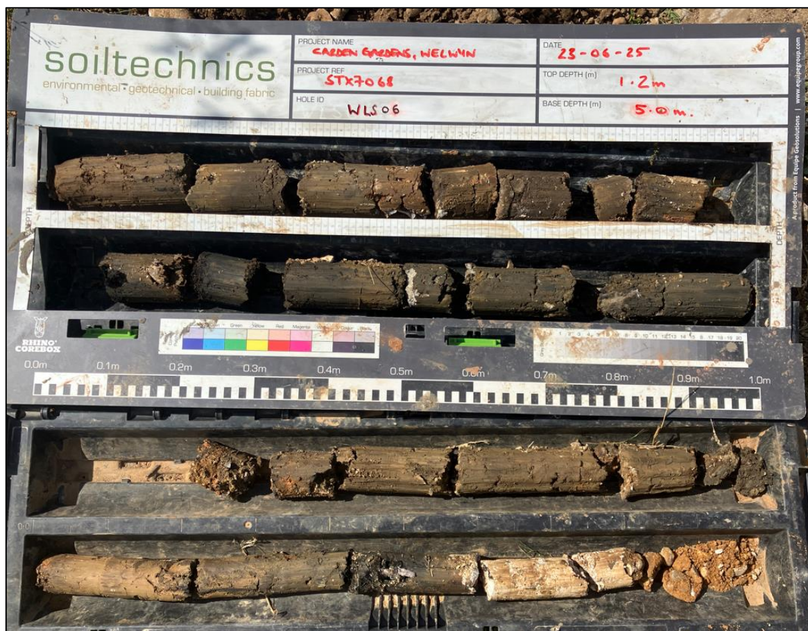
Figure 6-C: Fine-grained Made Ground encountered in WLS06 from 1.2m to 4.85m bgl.
