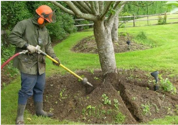
Figure A – Air Spade application
