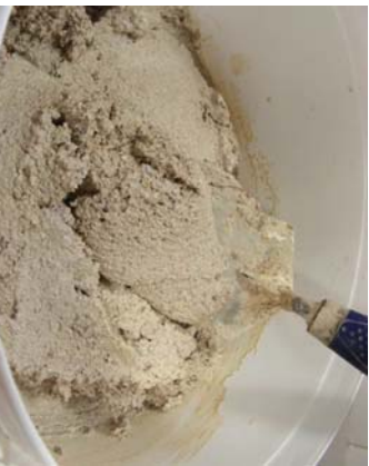
HISTORIC RANGE WALLS: LIME HAIR PLASTER FROM ANGLIA
