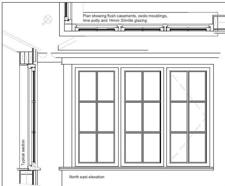
Extract from drawing 2420.07 showing flush casements, slim double glazing and less glazing bars
