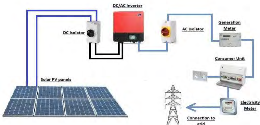
Figure 7 – Photovoltaic Panels – Typical Diagram
