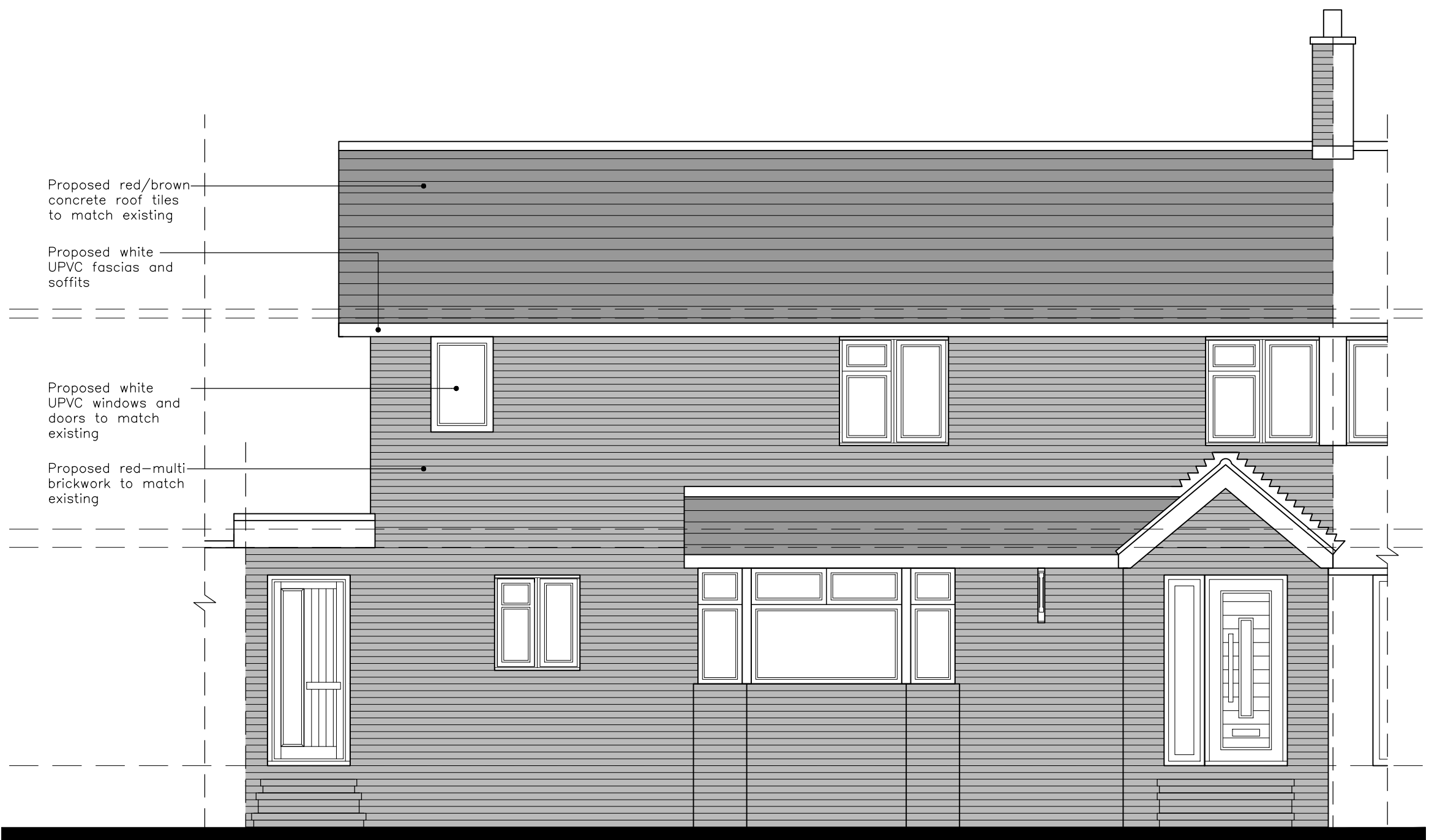
PROPOSED FRONT ELEVATION 1:50@A1
