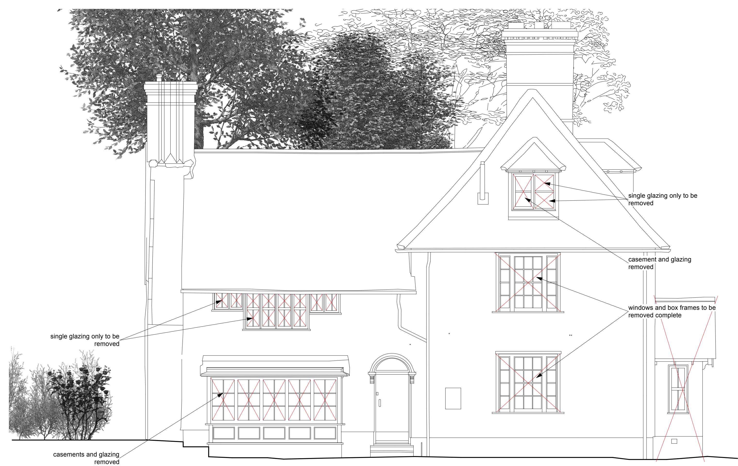
EAST ELEVATION AS EXISTING
