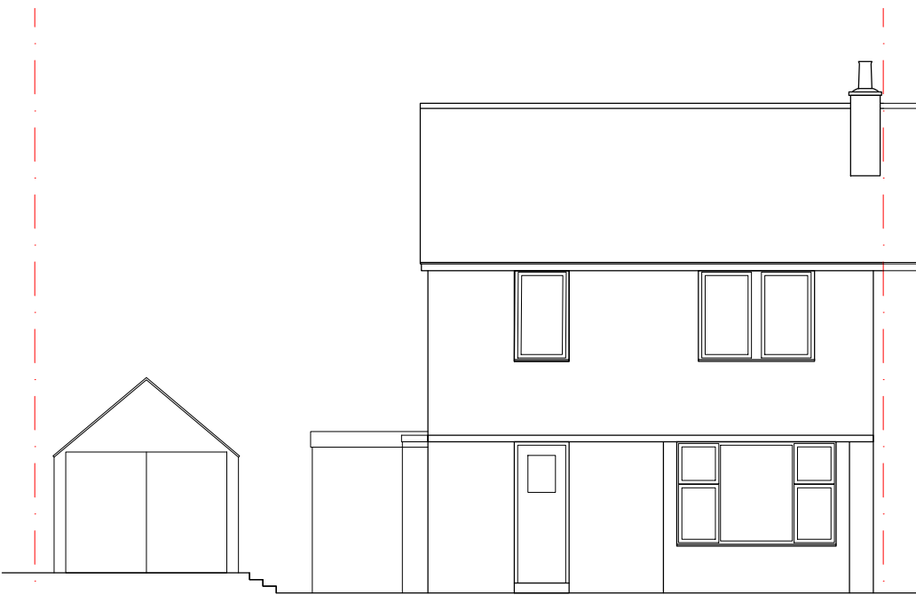
existing front elevation (SW) - scale 1:100
