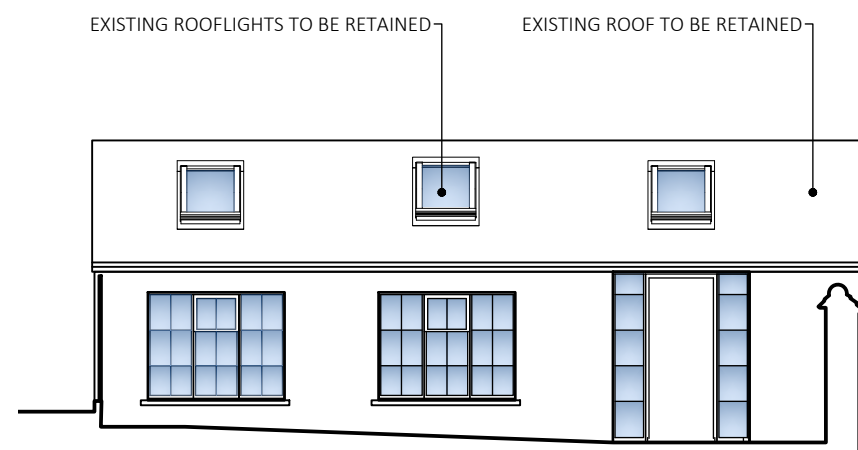
REAR ANNEX ELEVATION
