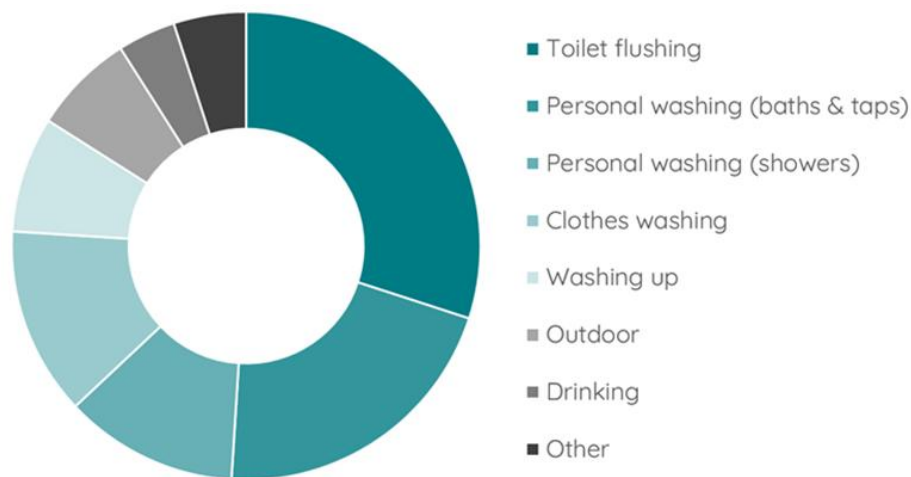
Figure 4: Domestic Water Consumption by End Use
