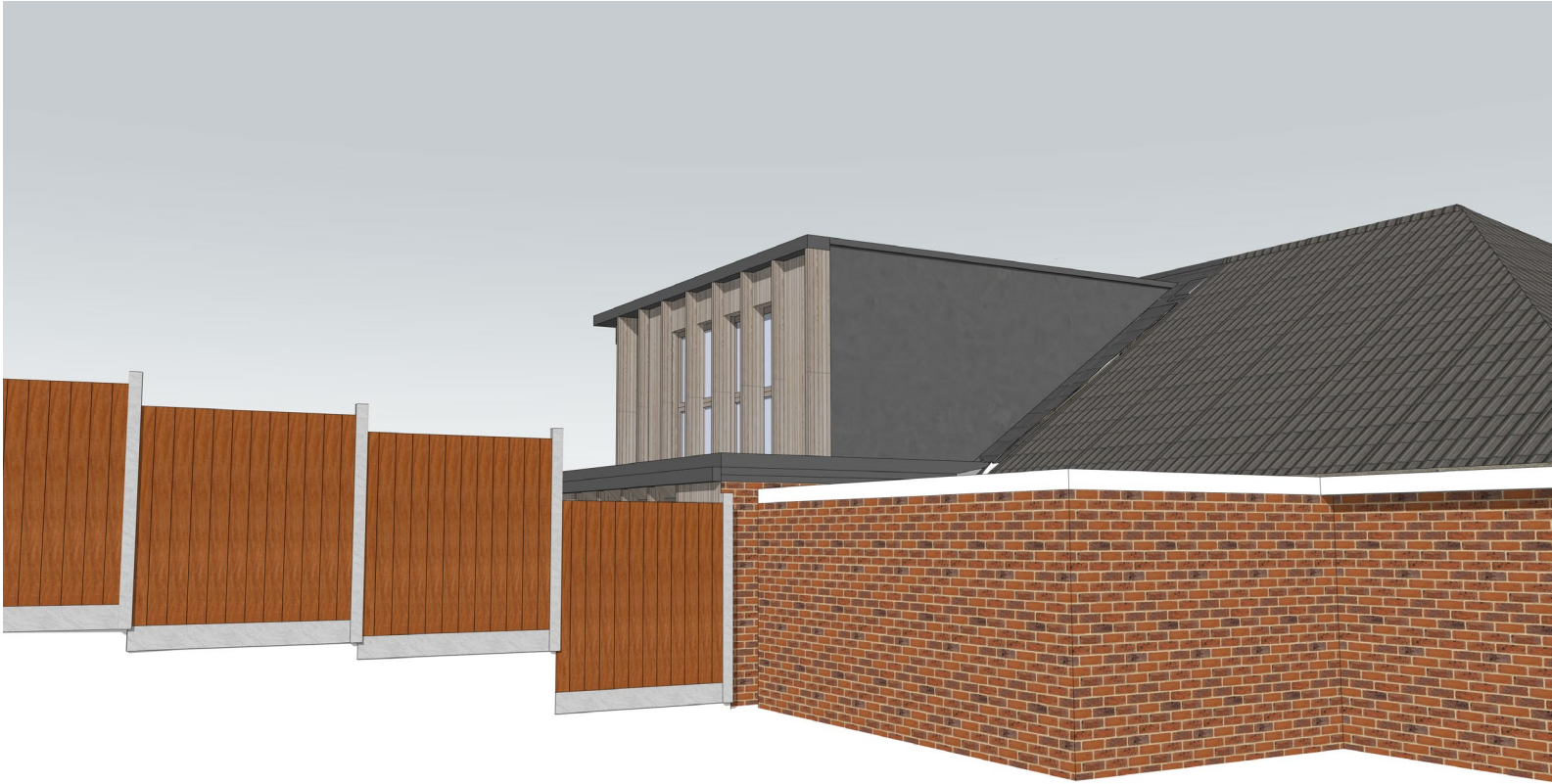
View from no. 29 garden, glazing is obscured by timber mullions
