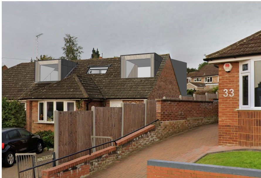
Updated elevation toward a consensus on the retention of the brick gable with their dormer expressed as a secondary element
