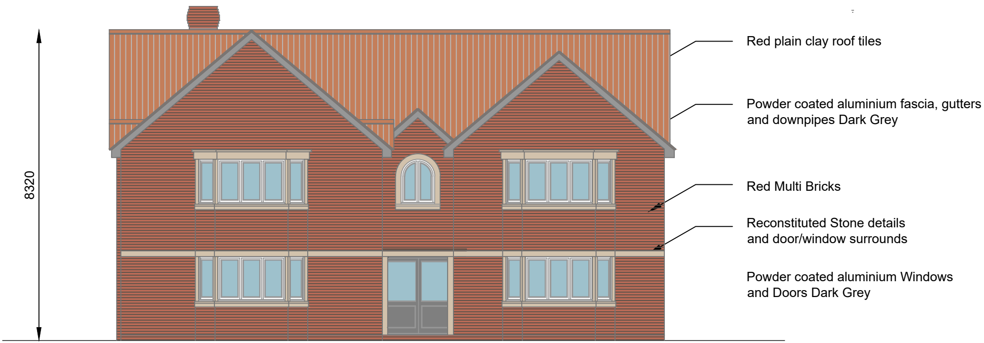
Front Elevation (West)
