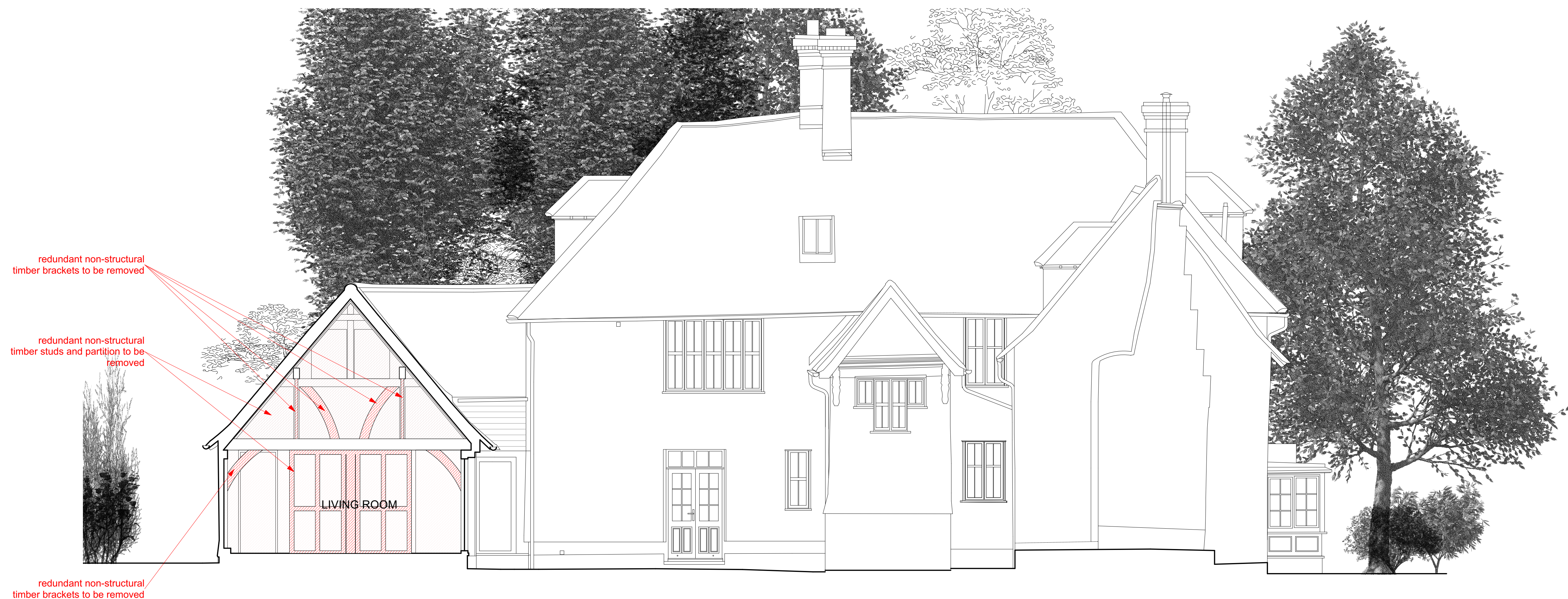
SECTION dd AS EXISTING showing proposed strip-out
