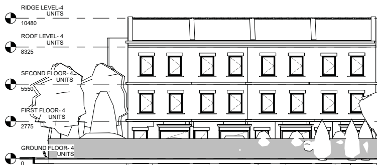
4 UNITS FRONT ELEVATION 1 : 100
