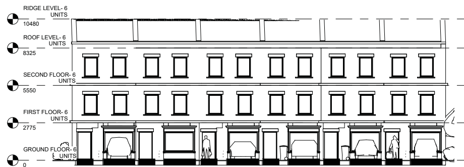
6 UNITS FRONT ELEVATION 1 : 100
