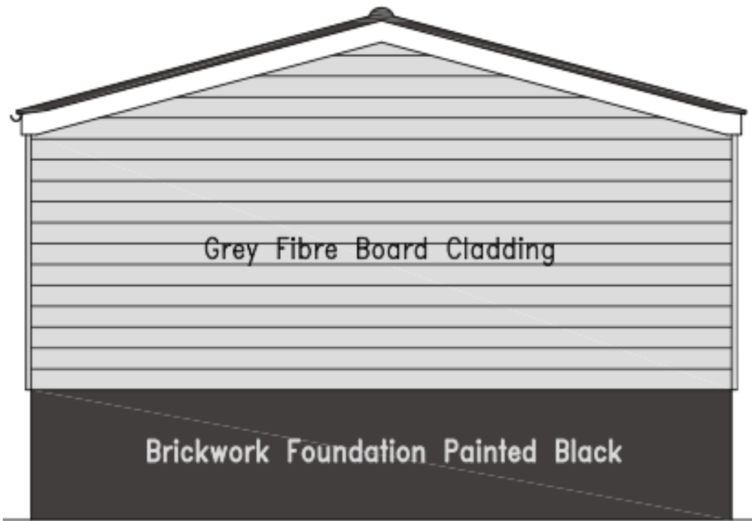
Figure 10. Replacement building south facing elevation
