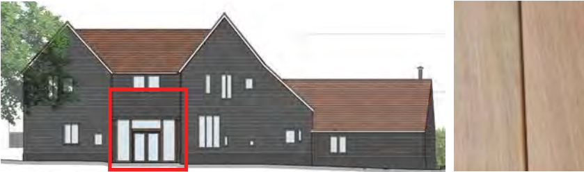
Proposed New Entrance Hall - proposed glazed link with oak framing and oak doors to contrast with main building
