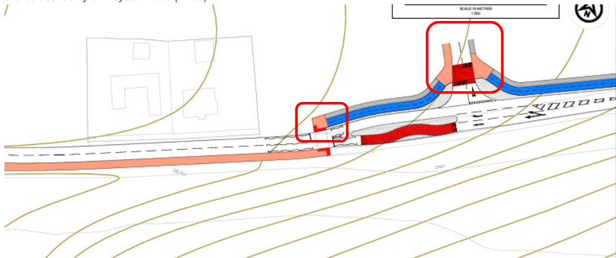
Image 20: Extract from PC7029-RHD-CE-GB-DR-D-0113 S3 I02, showing the lack of corduroy tactile paving at the extents of the shared-use facility on Royston Road (in red)
