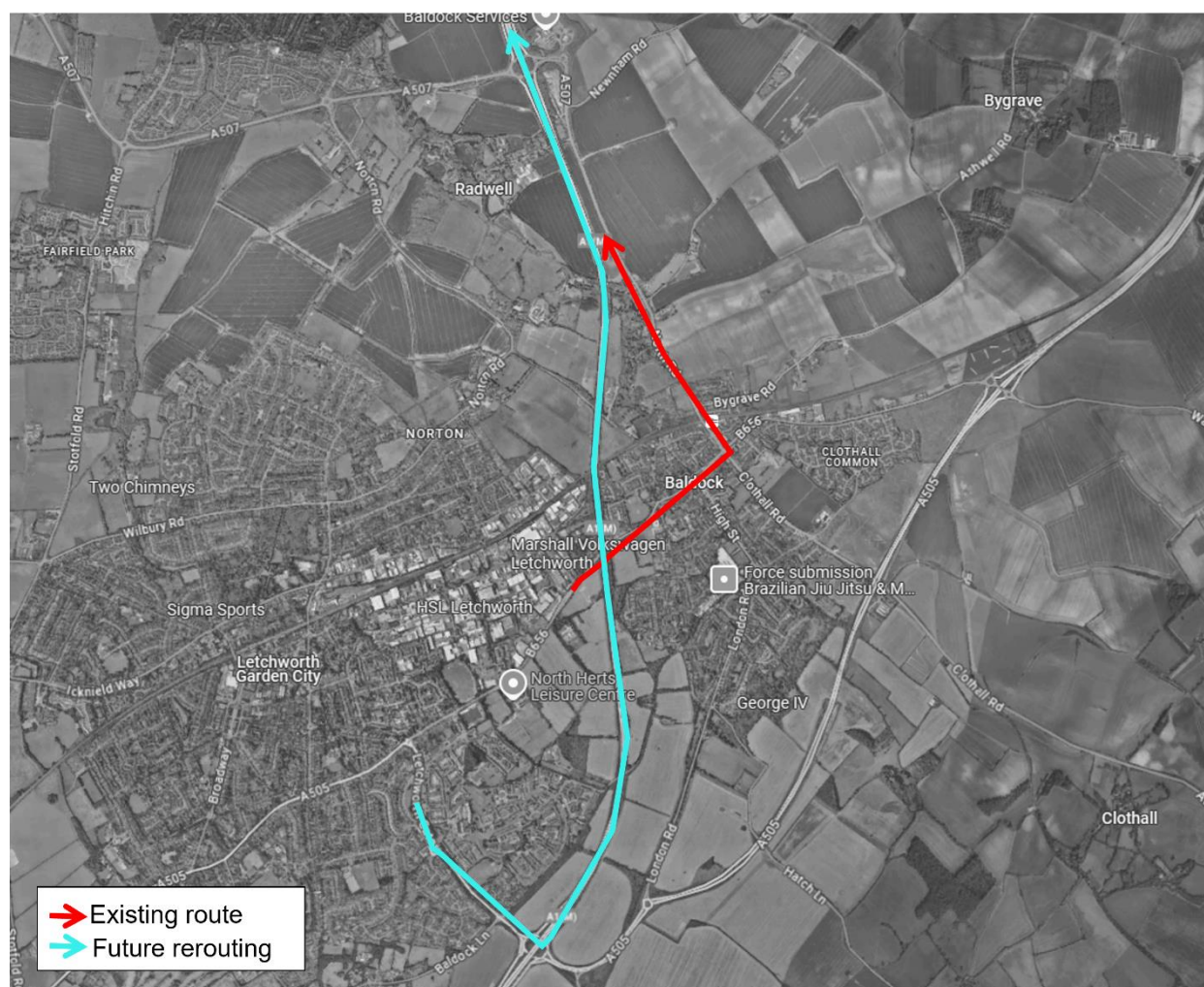
Figure 2-4: Whitehorse Street Left Turn Reassignment
