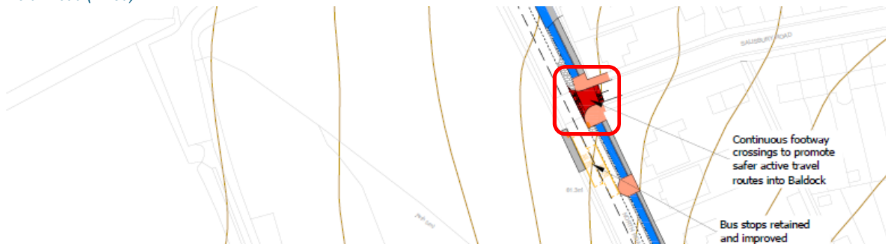
Image 11: Extract from PC7029-RHD-CE-GB-DR-D-0111 S3 I02, showing the lack of blister tactile paving at the crossing face on North Road (in red)
