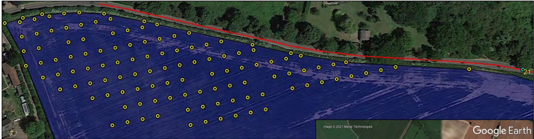
Figure 23 Reflecting area relevant to road receptor 21
