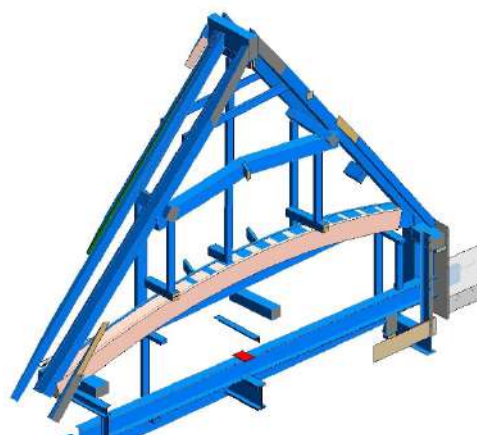
Figure 5. Measured survey showing timbers removed as part of 2022 works (but not agreed works)
