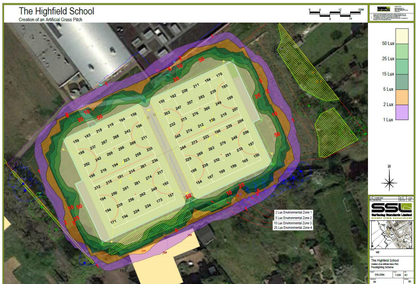
Figure 10 - showing the new artificial pitch and the floodlight contour plan overlaying aerial imagery. The floodlight mitigation has removed all light spillage onto the eastern boundary, and achieved the mitigation objective, although there is insufficient room to move the pitch to achieve the 25 metre buffer zone requested by best practice.
