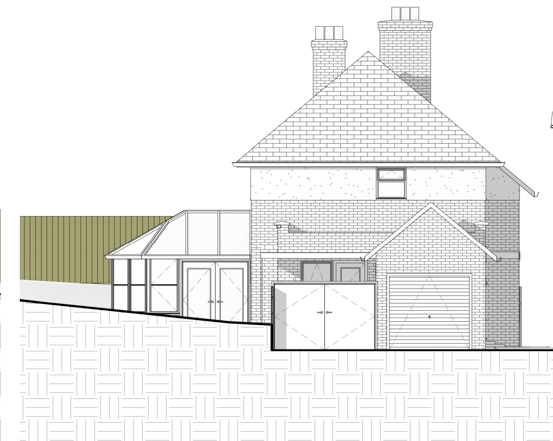
8 Side Elevation NE - As Existing 1 : 100
