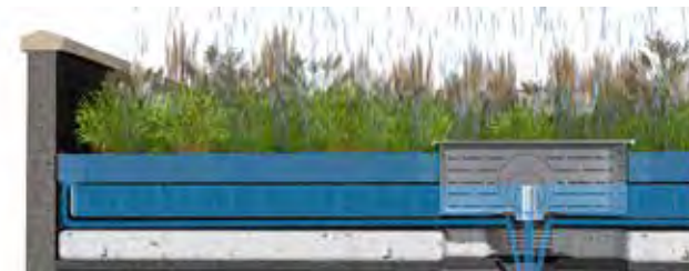
Fig.10.2. Blue roof drainage .
