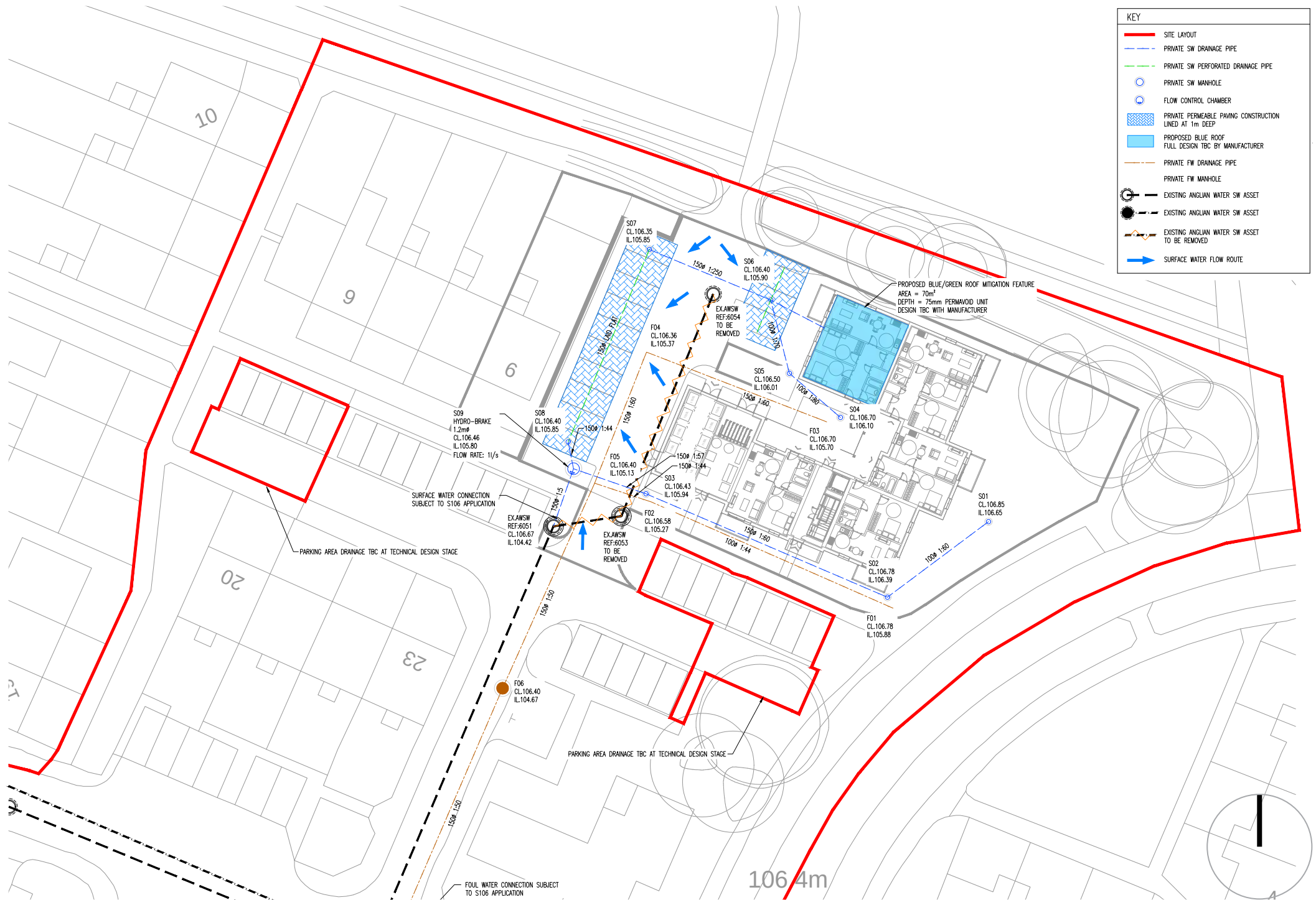
Fig. 11.2. Proposed drainage layout
