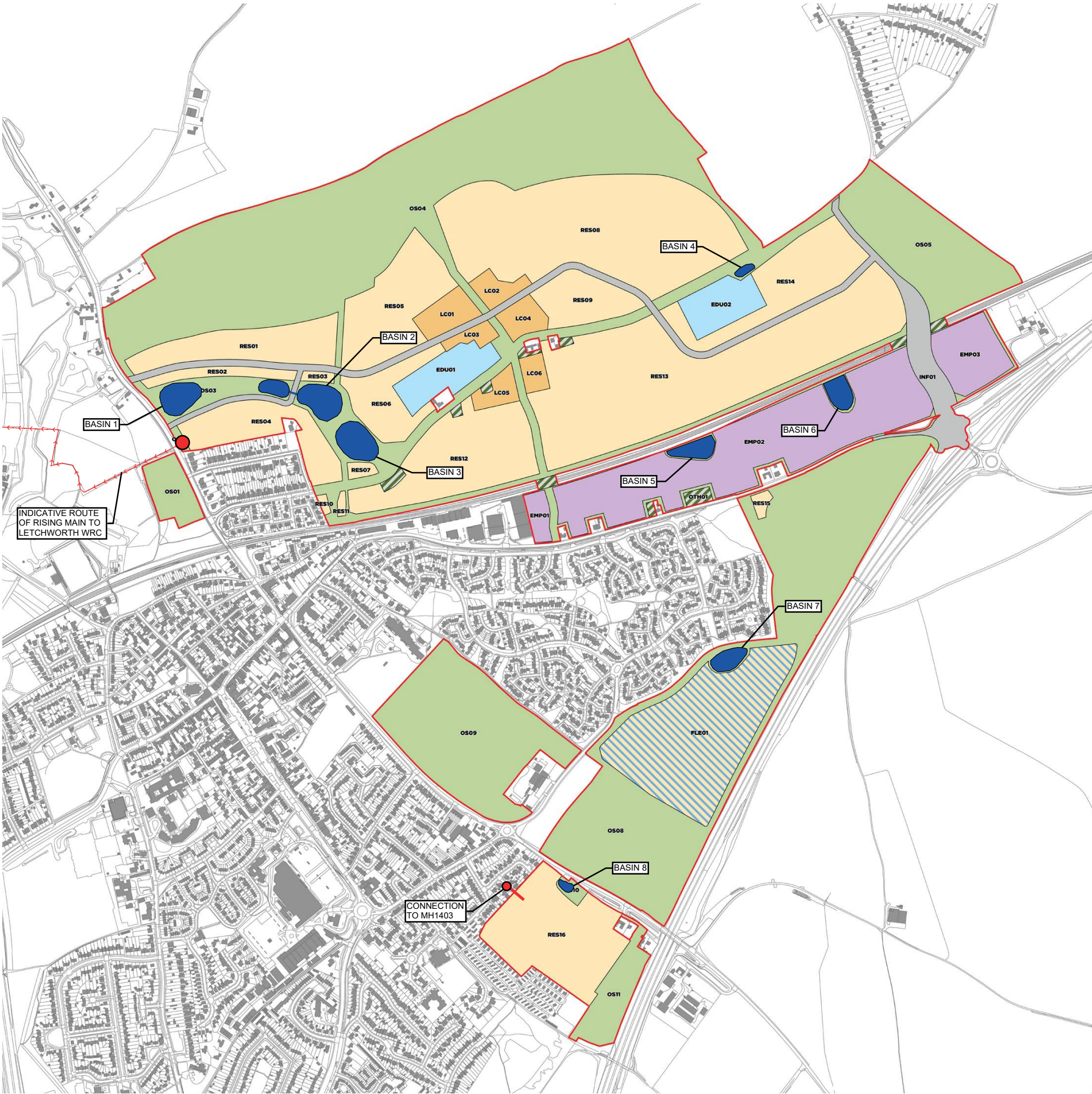
Figure 7.1 Infiltration basin and connection point locations
