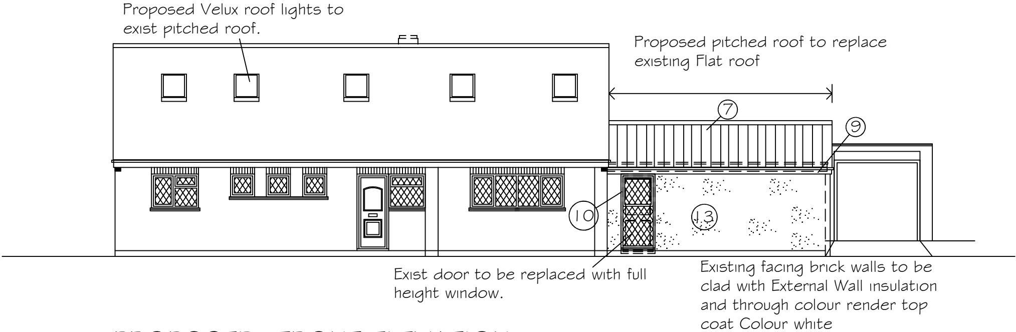
PROPOSED FRONT ELEVATION Scale 1:100
