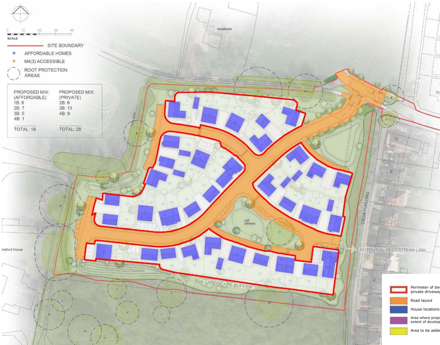
Diagram showing the road layout, house locations and private land perimeters of the approved site plan
