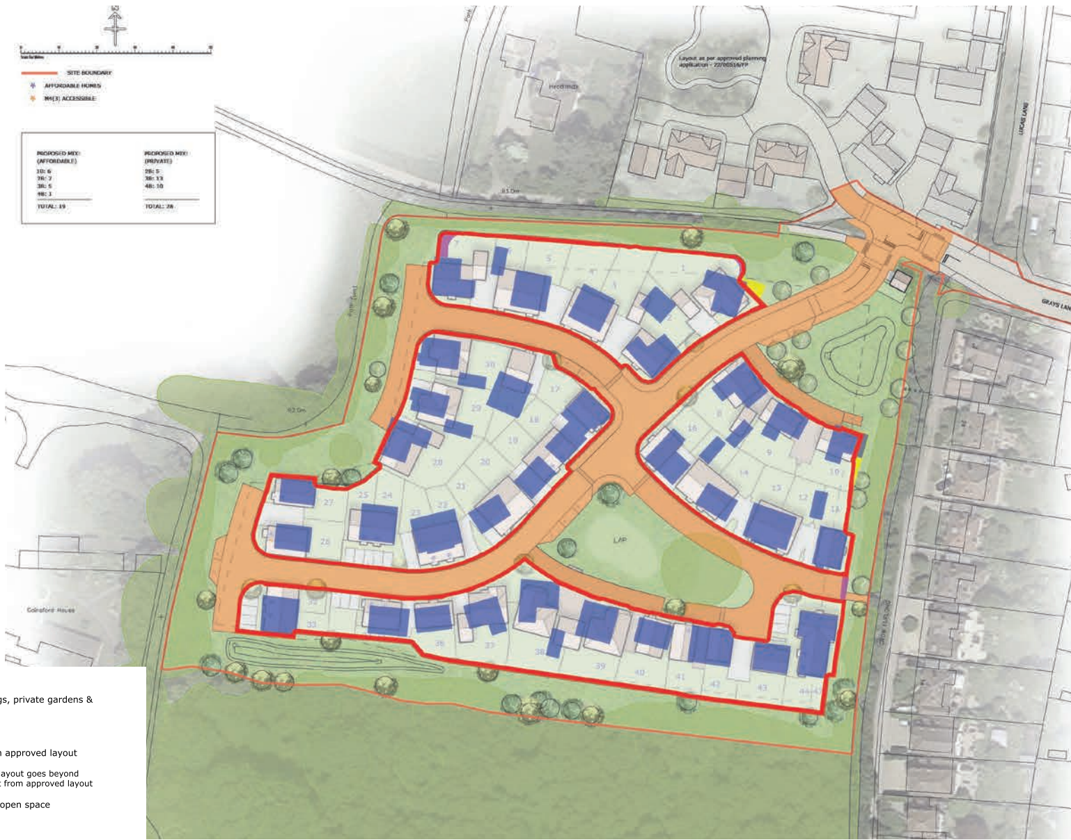
Diagram showing the road layout and private land perimeters of the proposed site plan plus the house locations from the approved layout.
