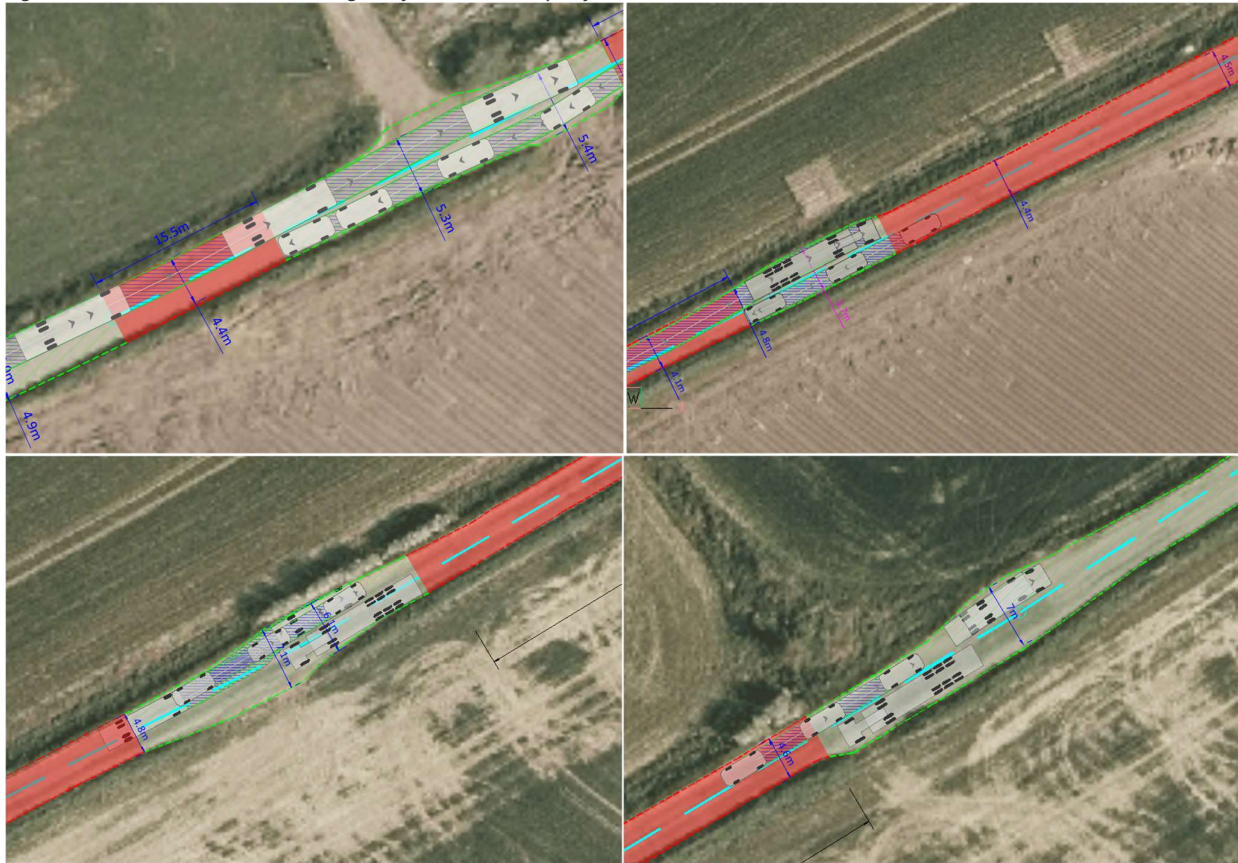
Figure 3-5: Section 2 – Vehicle tracking and forward visibility at four narrower sections
